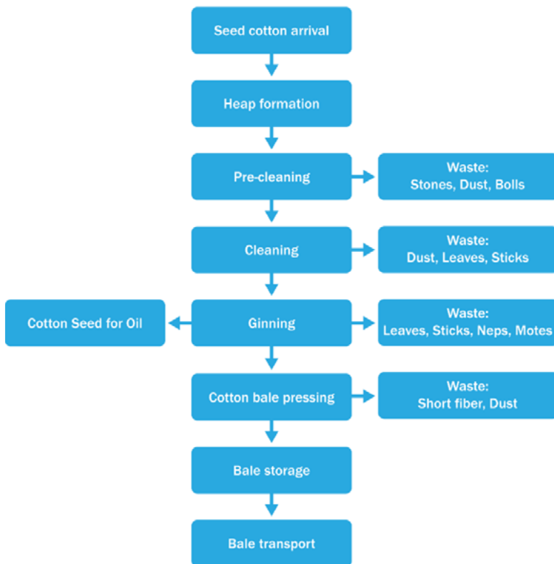
Figure 7: Material Flow in Ginning Unit
